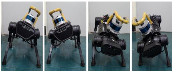
Figure 3. Examples of robot dog scanning postures
